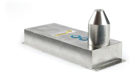
**Model M25:** 50 kV, 4W X-ray Monoblock - The M25 x-ray monoblock is a fully integrated miniature 50 kV, 4W x-ray generator designed specifically to be used as component of a handheld, portable, or benchtop x-ray instrument. The source includes a miniature sealed x-ray tube with a transmission-type end window, a high voltage power supply, and control electronics contained in a compact grounded enclosure.
