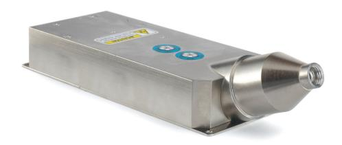
Model M47: 50 kV, 10W X-ray Monoblock - The M47 x-ray monoblock is a fully integrated miniature 50 kV, 10 W x-ray generator designed specifically to be used as component of a handheld, portable, or benchtop x-ray instrument. The source includes a miniature sealed x-ray tube with a transmission-type end window, a high voltage power supply, and control electronics contained in a compact grounded enclosure.
